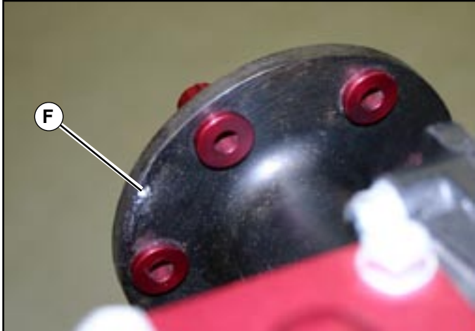
The dot stamped in the back of the prop hub's flange (F) will be in the position shown during initial timing. This view is from behind the engine.
