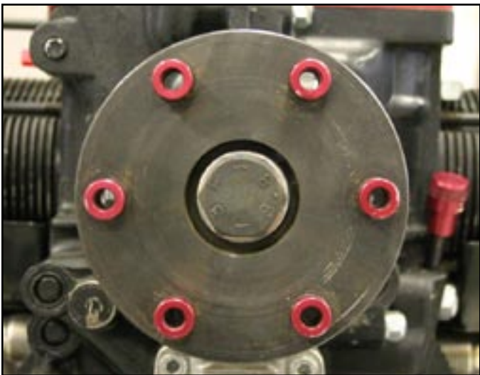
When the flywheel is properly positioned for static timing of the secondary ignition the prop bolt holes will be aligned as shown in this photo, and the stamped dot (F, top photo) will be positioned as shown in the top photo.
